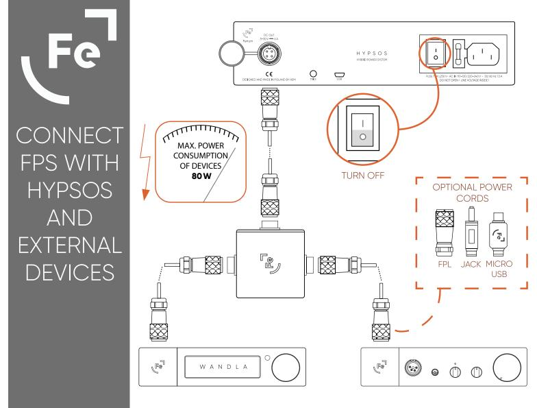
Set correct voltage values on HYPSOS before connecting Ferrum Power Splitter with external devices
